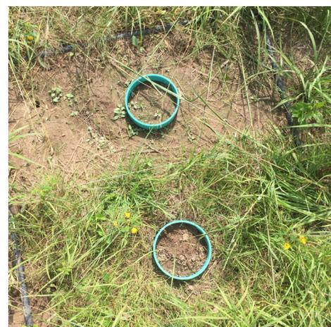
Top and bottom left: A gas analyzer in one of the prairie plots at Big Rock Valley was used to measure the rate at which carbon dioxide was released from the soil. Bottom right: Soil collars were used as a platform for the analyzer to rest upon so it did not directly touch the soil. (Researchers took measurements in the morning to avoid changes in flux as temperatures warmed.)
