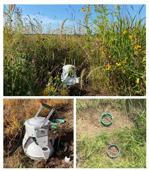
Top and bottom left: A gas analyzer in one of the prairie plots at Big Rock Valley was used to measure the rate at which carbon dioxide was released from the soil. Bottom right: Soil collars were used as a platform for the analyzer to rest upon so it did not directly touch the soil. (Researchers took measurements in the morning to avoid changes in flux as temperatures warmed.)
