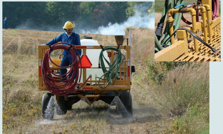
The War Wagon shown wetting a firebreak during a burn. (Inset) Three valves on rear of the trailer feed into a series of custom nozzles.
